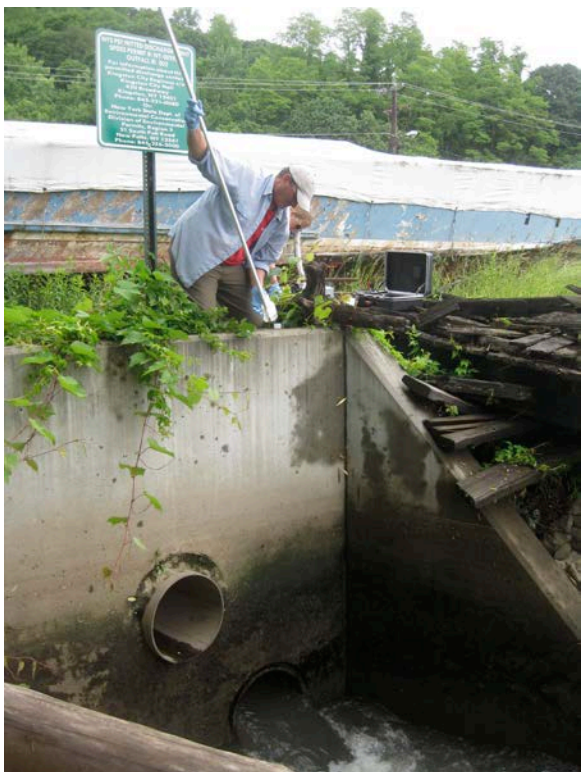
Figure 6. Sample collection at the Kingston WWTP CSO that empties into Rondout Creek.
