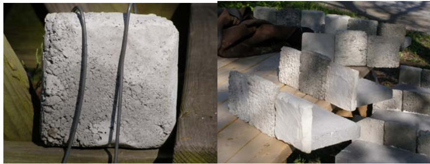
Figure 3: Tile stabilization structures. Wire anchors for sheltered sites (left) and concrete composites for exposed sites (right).
