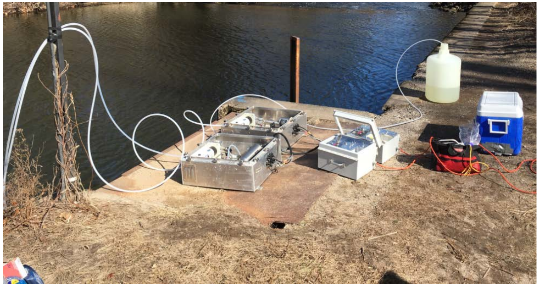
Figure 1. Trace Organics Platform Sampler (TOPS). Here two units are collecting duplicate samples of suspended solids and filtered water. The carboy in the upper right is collecting filtered water to determine the volume of water passed through the glass fiber cartridge. Aqueous samples for chemical analysis are pumped directly into laboratory cleaned glass jugs. Power is being supplied by portable generator.
