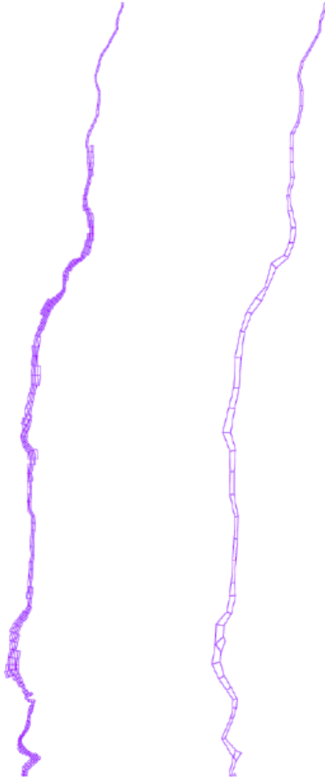
Figure 3-7. Hudson River, from Troy Dam to the head of Haverstraw Bay, view of CARP 127 x 205 (left) and 49 x 84 (right) model computational grids.
