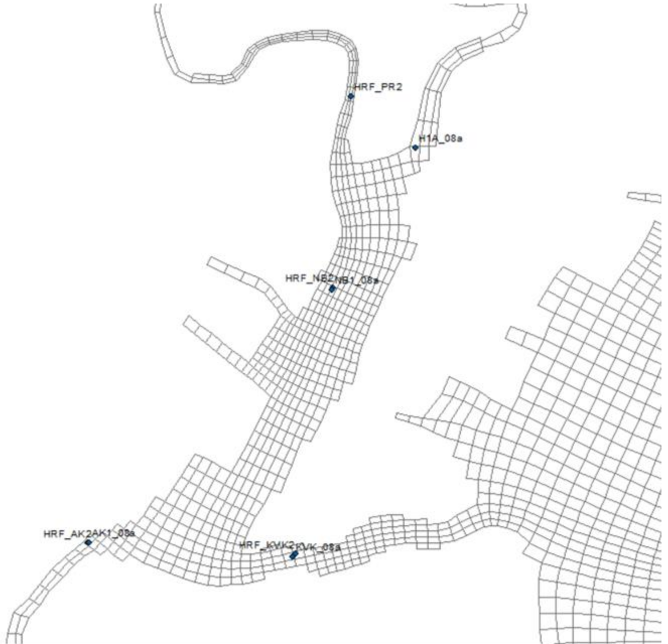
Figure 3-25. Locations of velocity currents model and measurement comparisons for 2007-09 water years imposed on 127 x 205 CARP model computational grid.
